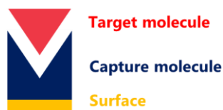
Figures 1 – Key elements of an SPR biosensor.
