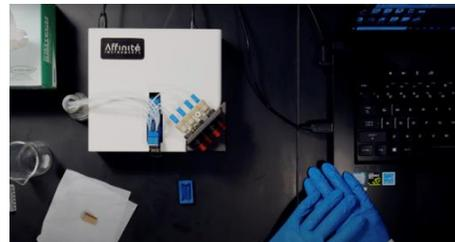
Affinité instruments P4SPR is a modular, label-free multichannel system with great application versatility. Its accessibility and ease of use allow for rapid high quality SPR results in antibodies characterization. Its multichannel feature increases result precision and additionally, with the Affinité manufactured sensors, non-specific interactions are greatly reduced. This would be especially interesting for studying interactions in crude samples.
