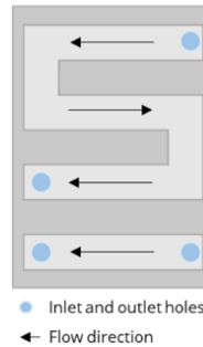
Figure 8 - P4SPR microfluidic cell design.
