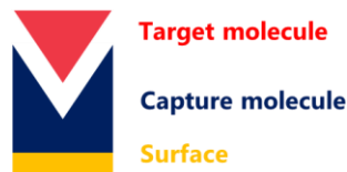
Figures 1 – Key elements of an SPR biosensor.
