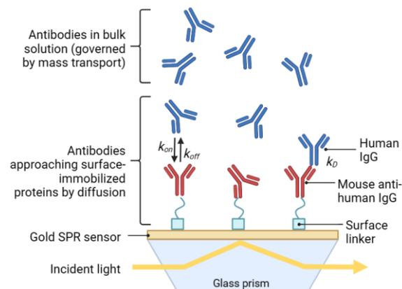
Fig. 3. Scheme of binding and molecular events.
