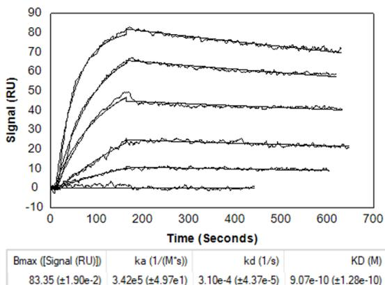
Fig. 7. Evaluation of kinetic parameters via TraceDrawer
