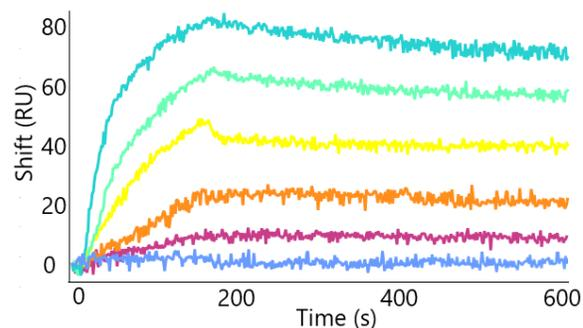
Fig. 6. Compilation of kinetic SPR sensorgram of Hm IgG of different concentrations (0, 0.89, 2.7, 8.0, 24, 72nM) binding with immobilized MAH IgG adjusted with reference channel and blank.
