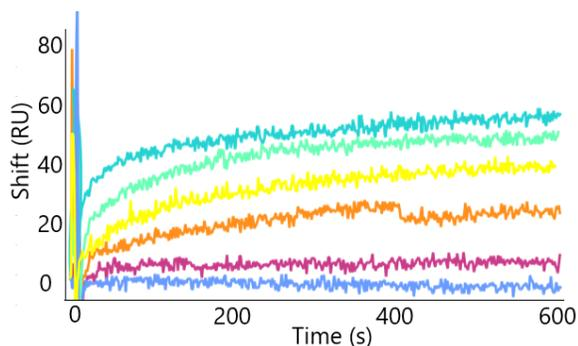
Fig. 4. Compilation of static SPR sensorgram of Hm IgG of different concentrations (0, 0.89, 2.7, 8.0, 24, 72nM) binding with immobilized MAH IgG adjusted with reference channel.
