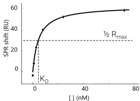
Fig. 5. Static evaluation of  $K_D$  in ezControl software obtained by plotting SPR shift in RU vs concentration in nanomolar.
